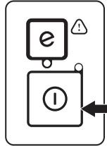
Press the power trigger lockout up. It is placed on the front handle.
