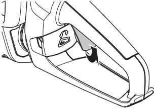
Release the power trigger and check thereby the free back movement of the power trigger. The cutting unit must stop within 1 second.
