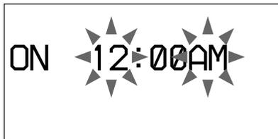
Press **↑/↓** to select the hour, and then press **→** so that the minute indication flashes. Do the same to set the minute. To go back to the hour indication, press **←**. When you press ENTER after setting the minute, "OFF" appears and the hour indication flashes.
