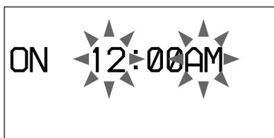
Press **↑/↓** to select the hour, and then press **→** so that the minute indication flashes. Do the same procedure to set the minute. To go back to the hour indication, press **←**. When you press ENTER after setting the minute, "OFF" appears and the hour indication flashes.
