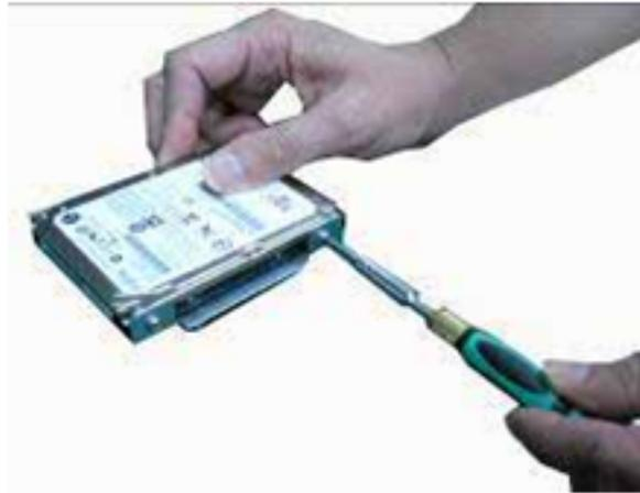
**Step 6** Install and fix the HDD through the side, next, plug the power cable in HDD.
