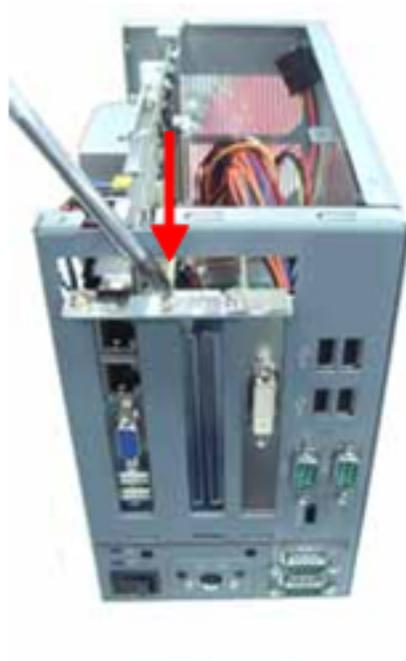
**Step 6** Close the top cover back to the chassis and fasten all screws.
