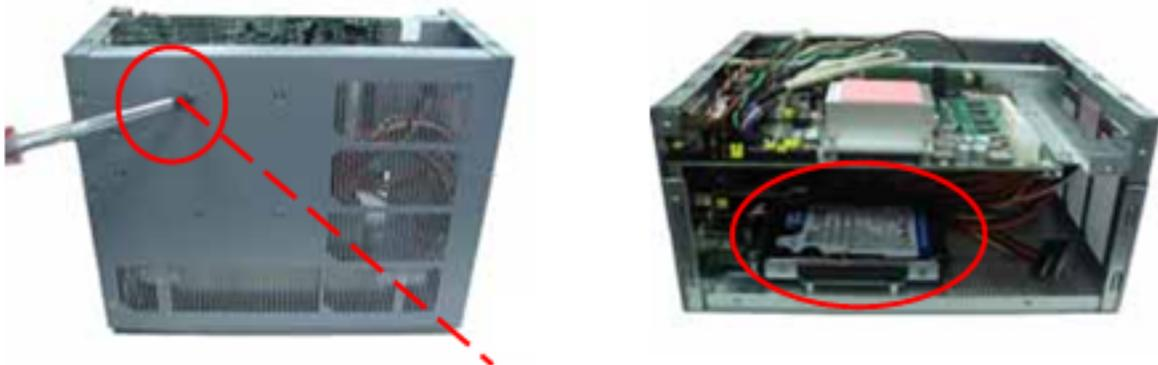
**Step 7** Close the top cover back to the chassis and fasten all screws.
