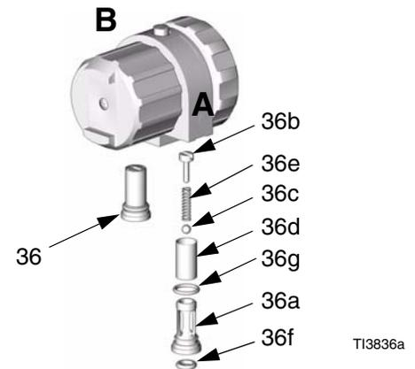
6. Reassemble check valves. Screw (36b) should be flush (within 1/16 in. or 1.5 mm) of housing (36a) surface. Liberally lubricate o-rings (36f, 36g) and carefully reinstall in fluid housing.
