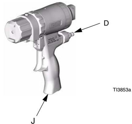
2. Attach fluid manifold. Connect air. Return gun to service.
