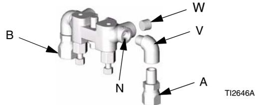
5. Connect A and B hoses to A and B swivels.
