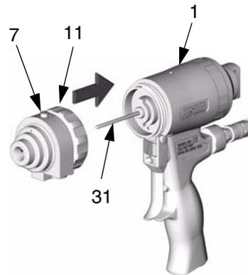
4. Push mix module (39) onto rod (31) as far as possible.
