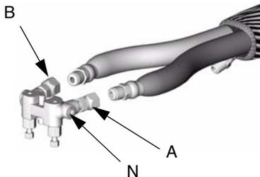
4. Apply thread sealant to plugs (W), elbows (V), and male threads of swivels (A, B). Install elbows (V) in optional inlets (N), facing down. Install swivels (A, B) in elbows. Be sure to install A swivel (smaller) in A side. Install plugs (W) where swivels had been. Torque all parts to 235-245 in-lb (26.6-27.7 N•m).
