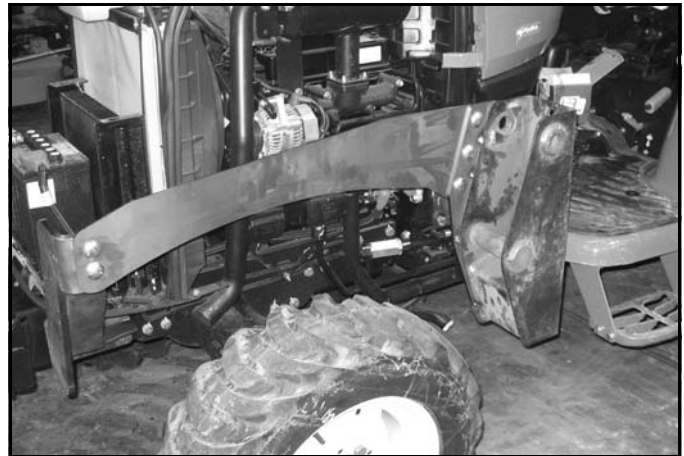
Figure 6. Left Side Rail Installed
