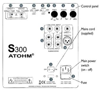
The subwoofer MUST be connected to the mains with the enclosed connector cord. The main switch has to be on "on" position and the (N°8) switch "on-auto-off" in the "auto" position. Your HF3 IP Subwoofer is equipped with a wide range of connection options for Hi Fi or Audi Video, Home Cinema.
