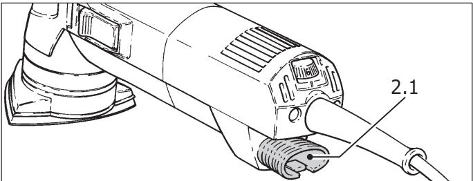
In order to draw off the dust produced during sanding the hose ( $\varnothing$  27 mm) of a Festool dust extractor is attached to the suction adapter (1.2)
