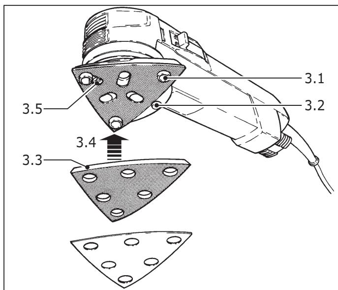
The sanding pad is made of MPE foam (micro-cellular polyurethane elastomer) and has bevelled edges (3.3). It has a velour fabric on its top surface and a Stickfix covering on its underside. The velour side of the sanding pad is pressed against the Stickfix covering of the sanding base (3.4). The tool's sanding base has three centring protuberances (3.1) at its corners enabling easy adjustment.
