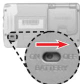
9. Wait five seconds, then switch the **Battery Switch** to **ON**.
