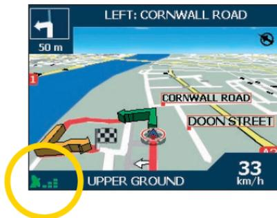
Tap the **GPS Strength Indicator** to open the *Satellite Signal Strengths* screen.
