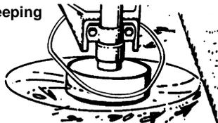
**EDGING** - Adjust trimmer to the edging position (see TWIST AND EDGE section). Allow only the tip of the line to make contact. Do not force trimmer line into work area.
