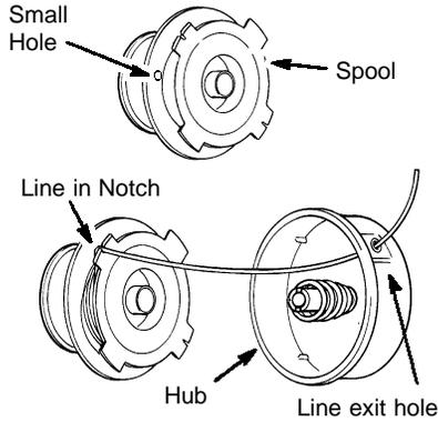
5. Wind the line evenly and tightly onto the spool. Wind in the direction of the arrow found on the spool.
