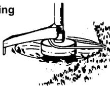
**SWEEPING** - The fanning action of the rotating line can be used for a quick and easy clean up. Keep the line parallel to and above
