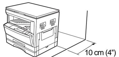
Be sure to allow the required space around the machine for servicing and proper ventilation.
