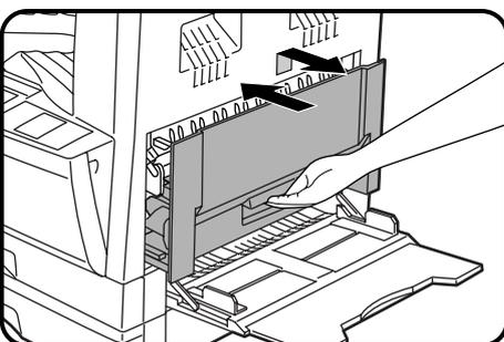
**3** Lift slightly on the side cover and slide the cover out until it stops. Close the side cover by pressing the handle on the cover.
