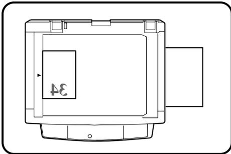
**2** Replace the first original with the second original and close the platen cover.
