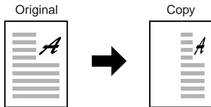
The XY ZOOM feature allows the horizontal and vertical copy ratios to be changed independently. This feature cannot be used with the 2 in 1 or 4 in 1 feature. (The 2 in 1 or 4 in 1 feature can only be used when an optional electronic sorting kit and an optional SPF are installed.)
