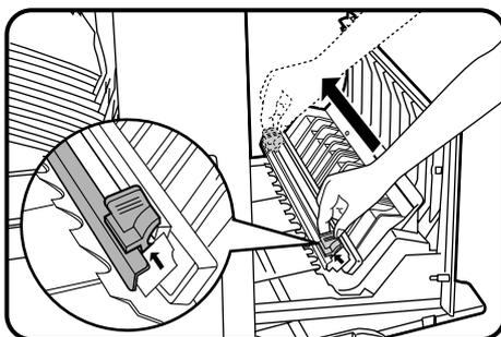
**4** Set the charger cleaner onto the transfer charger and gently slide the cleaner in the direction indicated by the arrow two or three times.
