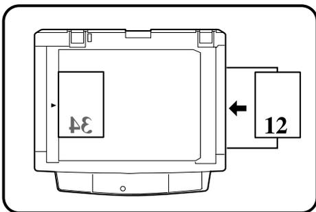
**3** Turn the first copy over left to right and place it into the bypass tray.
