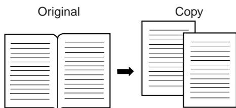
The DUAL PAGE COPY feature produces individual copies of two documents placed side by side on the original table. It is especially useful when copying books and other bound documents. This feature cannot be used with the 2 in 1 or 4 in 1 feature and sort/group feature. (The 2 in 1 or 4 in 1 feature and sort/group feature can only be used when an optional electronic sorting kit and an optional SPF are installed.) If the AUTO IMAGE feature has been selected, this feature cannot be selected.
