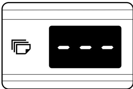
If the copier has been programmed in the auditing mode, “---” will appear in the copy quantity display in the initial conditions.
