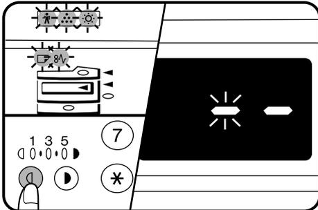
**1** Press and hold the light (Ⓛ) key for more than 5 seconds until all the alarm indicators (⚠, ⚡, ⚙, ☐, and ⚡) blink and “- -” appears in the copy quantity display.
