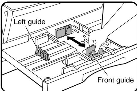
**3** Squeeze the lock lever of the front guide and slide the front guide to match the width of the paper.
