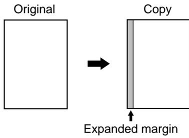
The MARGIN SHIFT feature automatically shifts the text or image to the right to increase the left margin by approximately 9 mm (1/4").
