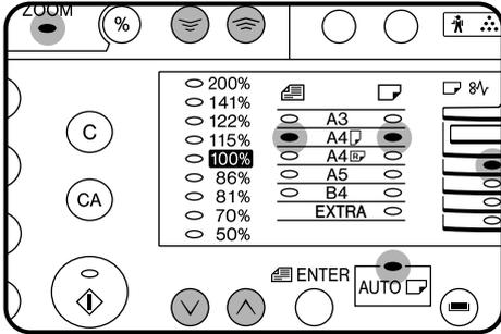
**5** Use the PRESET RATIO selector (⏴, ⏵) keys and zoom (⏴, ⏵) keys to change the copy ratio in the horizontal direction in a similar manner as for the vertical direction.
