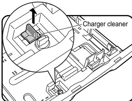
**3** Gently lift and pull out the upper paper tray and take the charger cleaner out by holding the tab.
