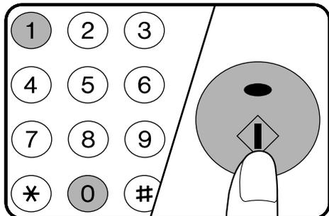
1. To reset an individual account, press the 0 key. To reset all accounts, press key 1.
