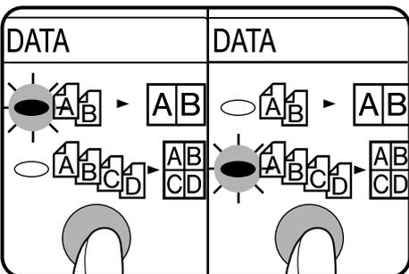
**3** To confirm or set the layout pattern for 2 in 1 copying, first ensure that both the 2 IN 1 (A<sub>B</sub> - A<sub>B</sub>) and 4 IN 1 (A<sub>B</sub>C<sub>D</sub> - A<sub>B</sub>C<sub>D</sub>) indicators are not lit then press and hold the 2 IN 1 / 4 IN 1 (A<sub>B</sub> - A<sub>B</sub>/A<sub>B</sub>C<sub>D</sub> - A<sub>B</sub>C<sub>D</sub>) key for more than 5 seconds.
