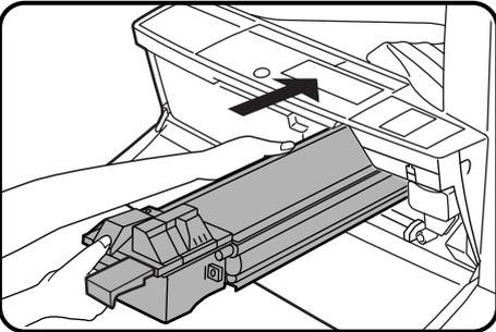
**5** Gently insert the toner cartridge along the guides until it locks in place while pushing the lock release lever.
