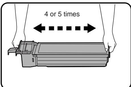
**4** Remove the new toner cartridge from the bag. Hold the cartridge on both sides and shake it horizontally four or five times.
