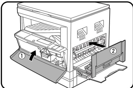
**7** Close the front cover by pushing both sides with your hands and then close the side cover by pressing the handle on the cover. The
