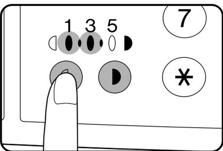
**3** Press the **light** (☐) or **dark** (◐) key to lighten or darken the automatic exposure level as desired.
