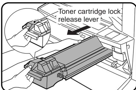
**3** Push the toner cartridge lock release lever and pull the toner cartridge out. Remove the toner cartridge while supporting it with the left hand at the green label position.
