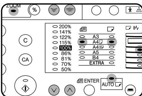
**3** Use the PRESET RATIO selector (⏏, ⏏) keys and zoom (⏏, ⏏) keys to change the copy ratio in the vertical direction.
