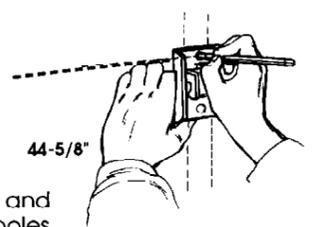
Remove bracket. If wall covering is ceramic tile, drill a 3/16-inch hole through tile only. Then proceed as follows:
