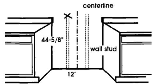
**3.** To mount anti-tip bracket to wood or metal wall stud: Find the wall stud that is closest to the center of the range location. (Note: Wall stud should **Not** be more than 12 inches to the right or left of center of range location.) Measure and mark at the center of the wall stud a distance of 44-5/8 inches up from the floor.
