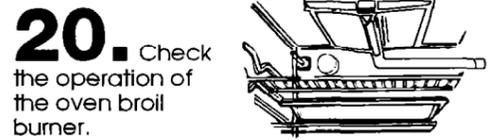
**20.** Check the operation of the oven broil burner. **If you have oven selector and temperature selector control knobs:** Turn the oven selector knob to "BROIL". Push in and turn the oven temperature selector knob to "BROIL". **The oven broil burner should light in 50 to 60 seconds. This delay is normal.** The oven safety valve requires a certain time before it will open and allow gas to flow.
