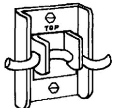
**7.** Push cable, located on rear of range, up and into the two hooks on the anti-tip bracket. Check that cable is secure in both hooks by pulling cable towards range. If cable comes out of hooks, reposition cable to insure that cable fits securely in both anti-tip bracket hooks. Slide range into final position.
