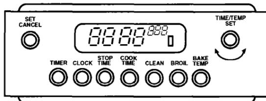
If you have electronic controls: Push "BAKE" button. °F will appear in the display. Turn Set knob until 350° appears in the display. **The oven burner should light in 50 to 60 seconds. This delay is normal.** The oven safety valve requires a certain time before it will open and allow gas to flow.
