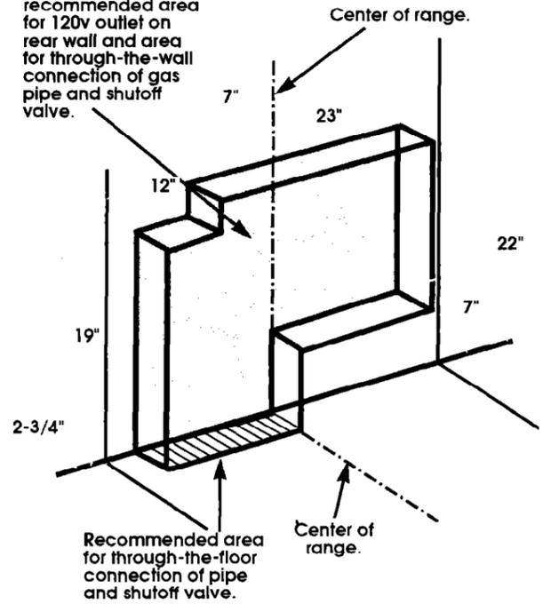
Recommended area for through-the-floor connection of pipe and shutoff valve.
