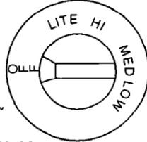
**15.** After burner lights, turn control knob to "HI" position. Check each cooktop burner for proper flame. At the "HI" setting, the small inner cone should have a very distinct blue flame 1/2" long. The outer cone is not as distinct as the inner cone. No air adjustment can be made.
