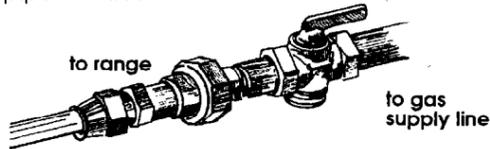
**F.** The supply line shall be equipped with an approved shutoff valve. This valve should be located in the same room as the range and should be in a location that allows ease of opening and closing. Do Not block access to shutoff valve.
