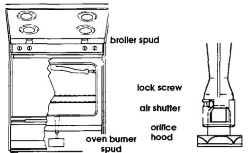
**19.** If oven flame needs to be adjusted, locate the air shutter near the center rear of the range. Loosen screw and adjust the air shutter until the proper flame appears. Tighten screw.
