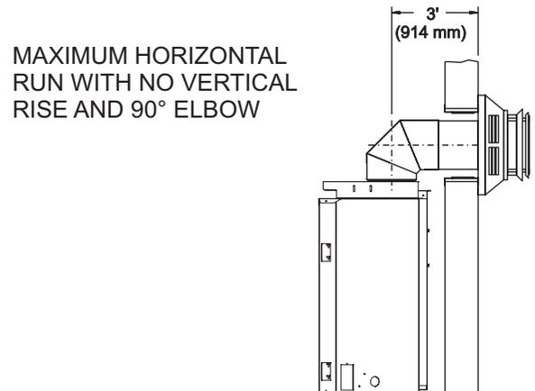
MAXIMUM HORIZONTAL RUN WITH NO VERTICAL RISE AND 90° ELBOW
