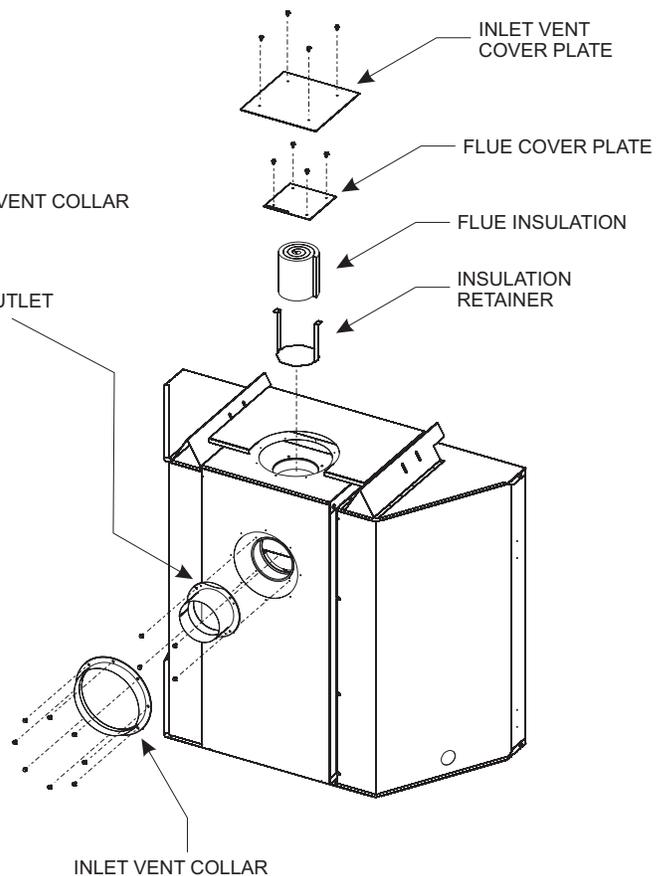
flue pipe before reinstalling the flue cover plate over the top flue with 4 screws.
