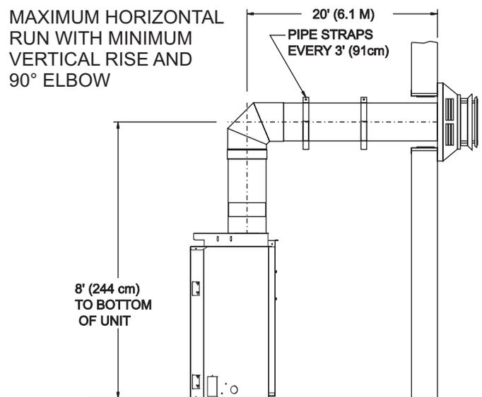
MAXIMUM HORIZONTAL RUN WITH MINIMUM VERTICAL RISE AND 90° ELBOW
