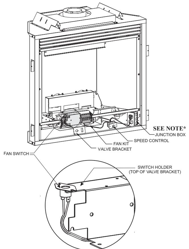
\*Note: Refer to Junction Box wiring instructions on page 68 for proper operation.
