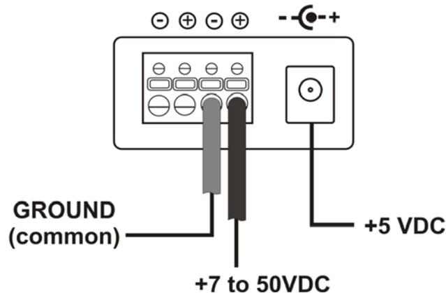
Connect the power source to any one positive and one negative terminal on the IE-ModeConverter.
