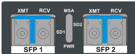
The IE-ModeConverter contains four status LED indicators. Each LED is dual color and has three states: off, red, or green. A loss of signal on one SFP causes the TX of the other SFP to turn off. This action does not activate the red TX Fault LED.
