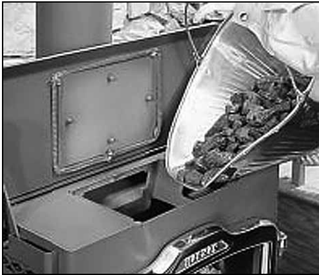
Add Even Layers by pouring evenly across coal bed
