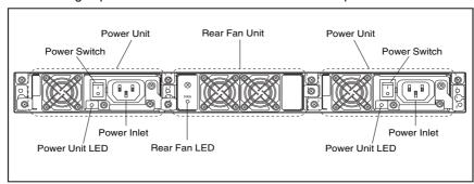
Power Switch Used to turn the XG700 on/off.
