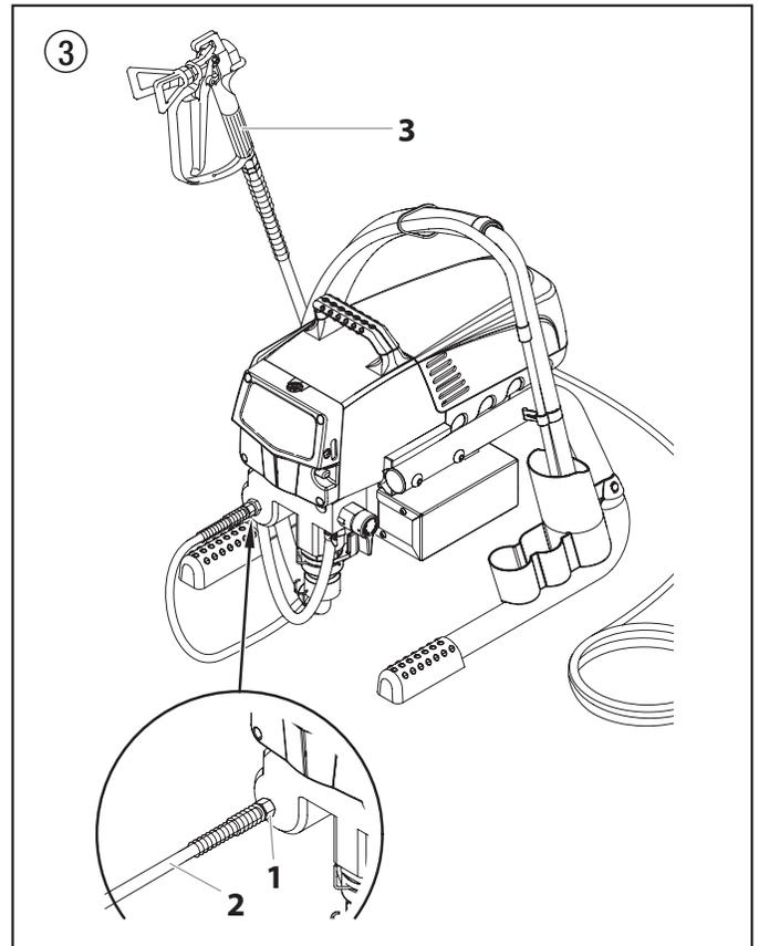
4. Remove the oil cup cap with a straight-slot screwdriver.
