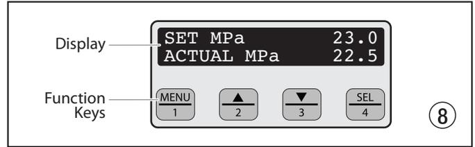
**i** The pressure control knob overrides the Digital Electronic Spray Control (DESC) settings. Anytime the pressure control knob is turned, the sprayer pressure will change accordingly.
