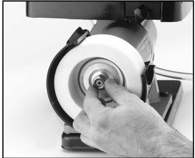
Figure 10. Removing dry wheel.
