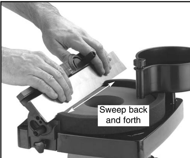
**Figure 7.** Grinding long knives.
