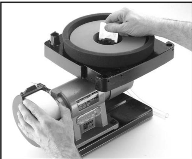
Figure 9. Removing wet wheel.
