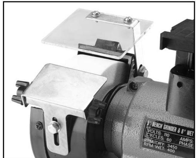
Figure 3. Dry wheel guard and rest positioning.
