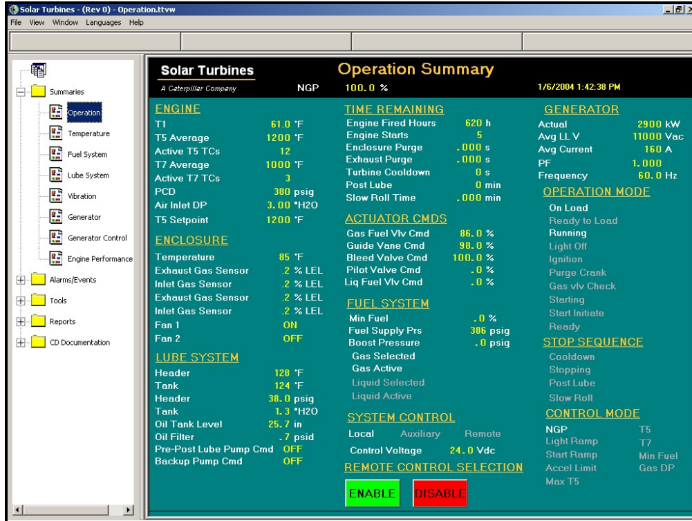
Figure 15. Typical TT4000 Operation Summary Display Screen
