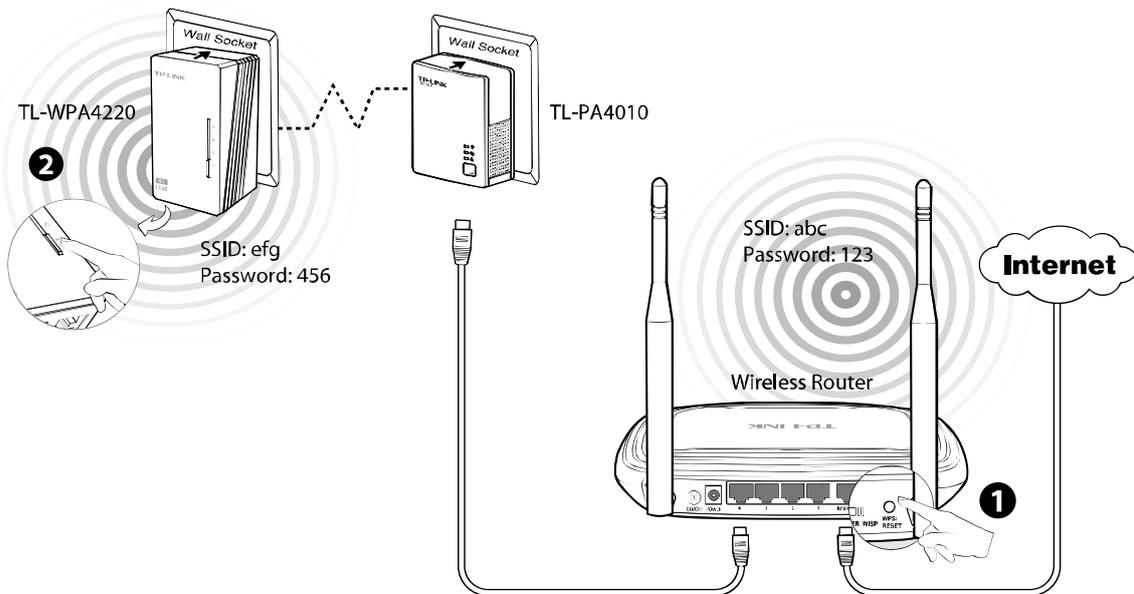
1. Press the WPS button on the router for 2 seconds. (Here we take TP-LINK router as an example.)
