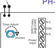
Relocking Time Delay Switch ensures the automatically turns to lock mode after the door is closed properly and it can be adjusted from 0 to 90 seconds.
