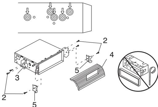
1. Select a position where the screw holes of the bracket and the screw holes of the main unit become aligned (are fitted) and tighten the screws at 2 places on each side.
