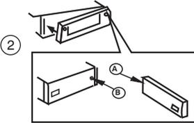
1. Attach the panel at the right side first, with point B on the main unit touching point A on the D.C.P. (As shown on the diagram).
