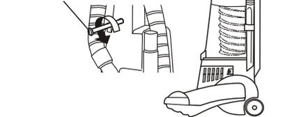
**3** Insert the screw that you removed. Be sure screw is tightened, but not over tightened.
