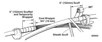
a. Insert base assemblies of shield connectors between the core wrapper and the shield  $180^{\circ}$  apart. Insert base assemblies of shield connectors between the core wrapper and the shield  $180^{\circ}$  apart. Install first nut and torque to  $45 \pm 5$  in-lbs ( $5.2 \pm 0.6$  kg·m).
