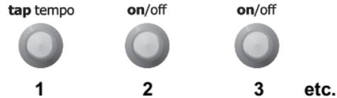
You can even scroll downwards using the foot switches: Press TAP TEMPO once, followed by one tap on the ON/OFF switch. Then press the TAP TEMPO switch again on or more times. Now you scroll downwards through the preset list.
