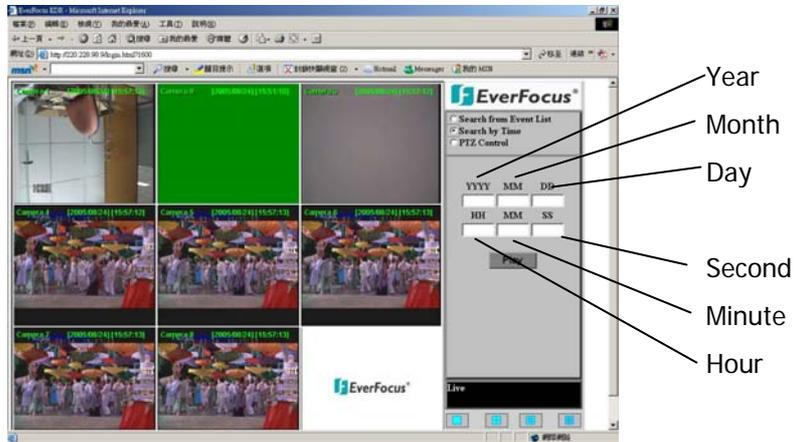
Selecting "Search by Time" opens an entry mask for playback position date and time input. Press the **PLAY** key to start the playback after data input.
