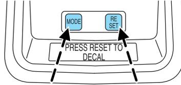
4. Press the RESET button to de-calibrate the compass. The display will read CIRCLE SLOWLY TO CALIBRATE for a few seconds and then display a direction with CAL displayed on the right side.
