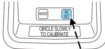
6. Slowly drive the vehicle in a circle (less than 3 mph [5 km/h]). This will take up to three circles to complete calibration.
