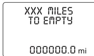
The DTE function will display LOW FUEL LEVEL and sound a tone for one second when you have approximately 50 miles (80 km) to empty. If you RESET this warning message, this display and tone will return within 10 minutes or 10 miles (16 km).
