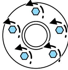
6. If equipped with a full wheelcover, remove the wheelcover center ornament then loosen the five black plastic nuts which retain the wheelcover using the lug wrench.
