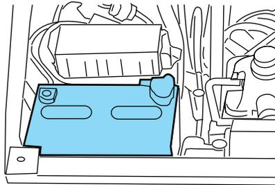
However, for severe usage or in high temperature climates, check the battery electrolyte level. Refer to *scheduled maintenance information* for the service interval schedules.
