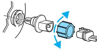
5. Without turning, remove the old bulb from the lamp assembly by gently pulling it straight back out of the lamp assembly.
