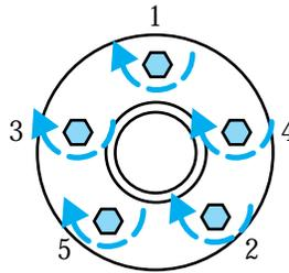
12. For full size spare aluminum wheel, firmly install the center ornament. If equipped with a full size spare tire/wheel assembly and lug nut retained full wheelcover, install the wheelcover by tightening the five black plastic nuts in the order shown on the wheelcover using the lug wrench with about 80 lb. in. (9 N•m) torque. Then firmly install the wheelcover center ornament.
