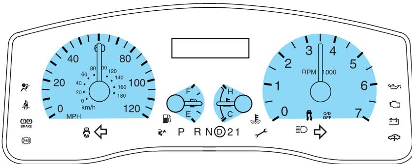
**Speedometer:** Indicates the current vehicle speed.
