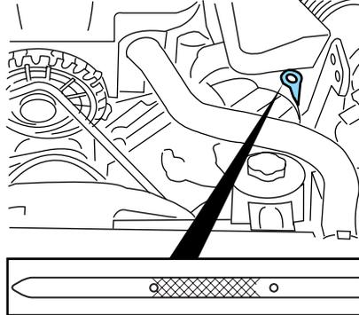
6. Wipe the indicator clean. Insert the indicator fully, then remove it again.
