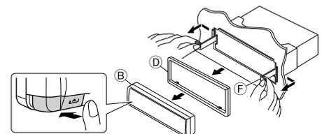
\*1 When you stand the unit, be careful not to damage the fuse on the rear.
