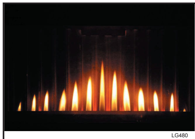
Fig. 35 Correct DVR28 flame. Center flame should be approximately 5½" (140 mm) high.
