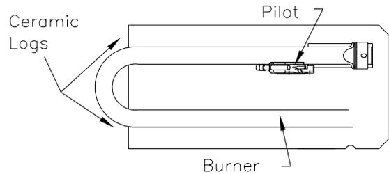
TOP VIEW OF BURNER ASSEMBLY
