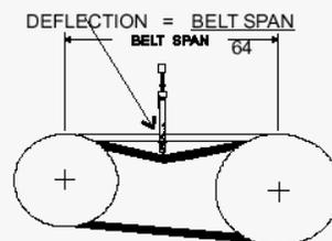
The capacity of the BROWNING® belt tension checker is 35 lbs. Other means of applying force must be used if force requirement is greater than this.
