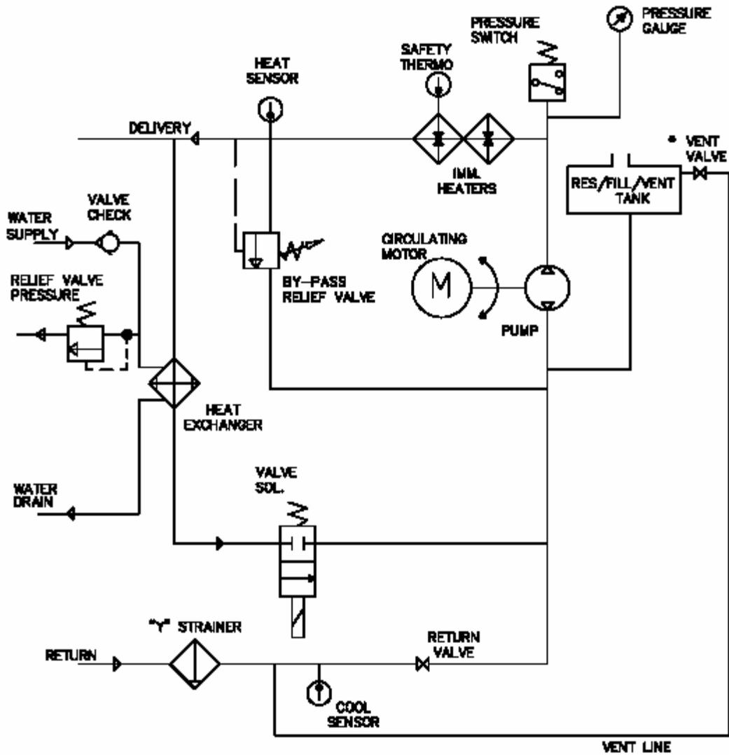
Note: The heat exchanger is optional, and the "Vent Valve" is also known as the "Blow-Off Valve."
