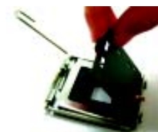
Fig. 2 Remove the plastic covering on the CPU socket.
