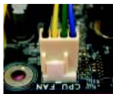
Fig. 6 Finally, please attach the power connector of the heatsink to the CPU fan header located on the motherboard.
