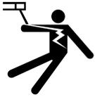
3.a. The electrode and work (or ground) circuits are electrically "hot" when the welder is on. Do not touch these "hot" parts with your bare skin or wet clothing. Wear dry, hole-free gloves to insulate hands.
