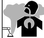
5.a. Welding may produce fumes and gases hazardous to health. Avoid breathing these fumes and gases. When welding, keep your head out of the fume. Use enough ventilation and/or exhaust at the arc to keep
