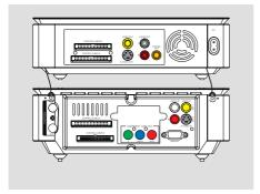
Connect the two ground cables fixed at the bottom of the DVD recordable player to the ground (<u>↓</u>) terminals on the rear of the HDD. Then, fasten the screws as shown to ensure firm connection.
