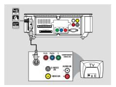
These connections enable you to watch and record TV programs using this recorder. If the antenna signal is connected via a VCR, Cable Box or Satellite Receiver, ensure that these devices are turned on in order to watch or record the cable programs.
