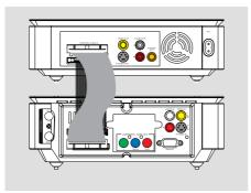
Connect the terminals marked CONTROL CABLE A and CONTROL CABLE B on the rear of the micro recordable theatre to the corresponding terminals on the rear of the power amplifier with the supplied 40pin and 36-pin IDE flat control cables by matching the pins.
