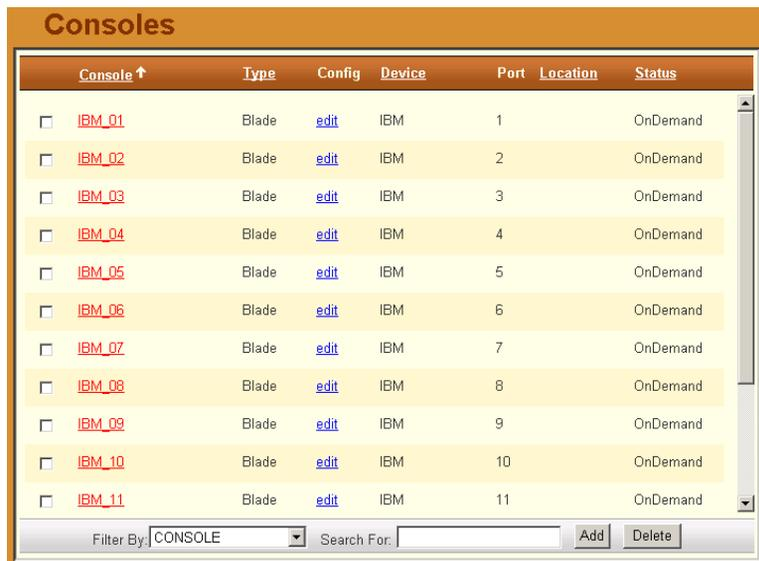
The screenshot shows a web interface titled "Consoles" with a table listing 11 blades. Each row includes a checkbox, a name (e.g., IBM\_01), a type (Blade), a configuration link (edit), a device (IBM), a port number (1-11), a location, and a status (OnDemand). At the bottom, there is a filter dropdown set to "CONSOLE", a search input field, and "Add" and "Delete" buttons.
