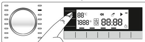
Press the **Temperature Adjustment** button to change the temperature. Temperature will decrease by increments of 10 °C.
