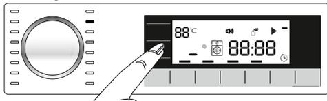
If you want to discharge the water at the end of the programme without spinning, use **No Spin** function.
