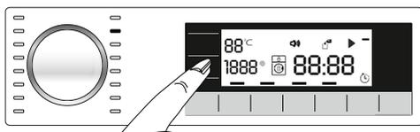
Press the **Spin Speed Adjustment** button to change the spin speed. Spin speed decreases gradually.
