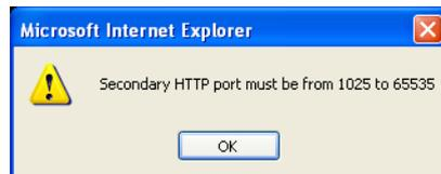
To access the Network Camera on the LAN, both the HTTP port and secondary HTTP port can be used to access the Network Camera. For example, when the HTTP port is set to 80 and the secondary HTTP port is set to 8080, refer to the list below for the Network Camera's IP address.
