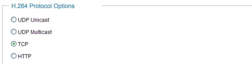
The screenshot shows a web interface for H.264 Protocol Options. It contains four radio button options: UDP Unicast, UDP Multicast, TCP, and HTTP. The TCP option is selected, indicated by a filled circle next to it.
