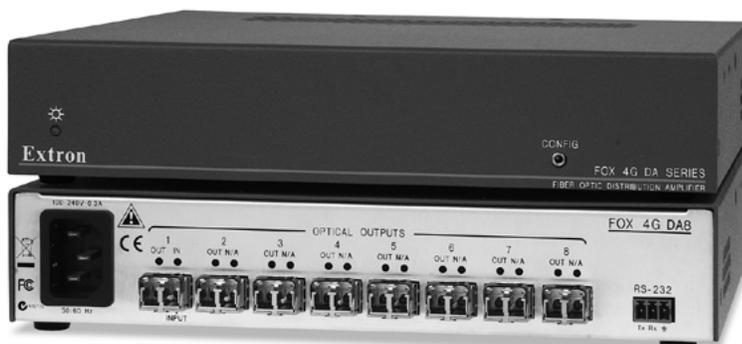
The Extron FOX 4G DA8 is an eight output fiber optic distribution amplifier for distribution and long haul transmission of fiber optic A/V and RS-232 control signals over a single fiber. Engineered for reliability and exceptional performance, it supports up to 4.25 Gbps digital distribution for standard definition video, high resolution computer-video, DVI-D, and multi-rate SDI. The FOX 4G DA8 also includes a host of features for enhancing A/V system integration.
