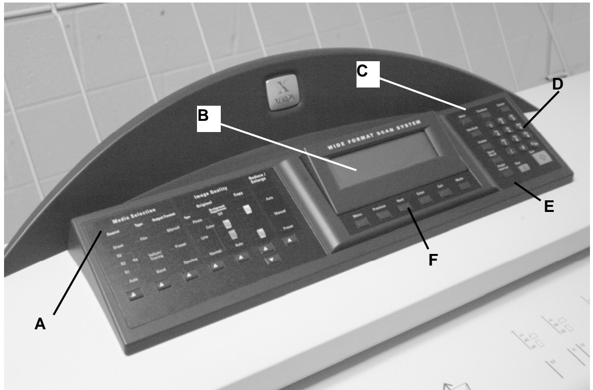
Scan System Control Panel
