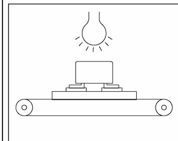
Reflow soldering under inadequate soldering conditions may result in unreliable relay performance or even physical damage to the relay (even if the relay is of surface mount type with high heat resistance).
