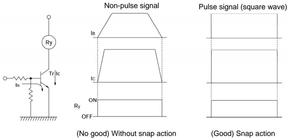
**4. Schmitt circuit (Snap action circuit) (Wave shaping circuit)**
