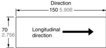
Also, as shown in the drawing below, when the pattern has a connector section, the direction is taken as shown by the arrow in the longitudinal direction.
