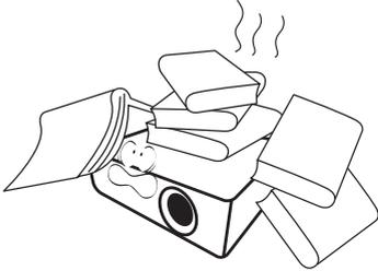
18. Do not place liquids near or on the projector. Liquids spilled into the projector may cause it to fail. If the projector does become wet, disconnect it from the power supply's power outlet and call BenQ to have the projector serviced.
