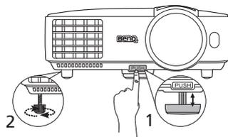
To retract the foot, hold up the projector while pressing the quick-release button, then slowly lower the projector. Screw the rear adjuster foot in a reverse direction.
