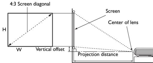
The screen aspect ratio is 4:3 and the projected picture is 4:3
