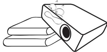
16. Do not stand the projector on end vertically. Doing so may cause the projector to fall over, causing injury or resulting in damage to the projector.
