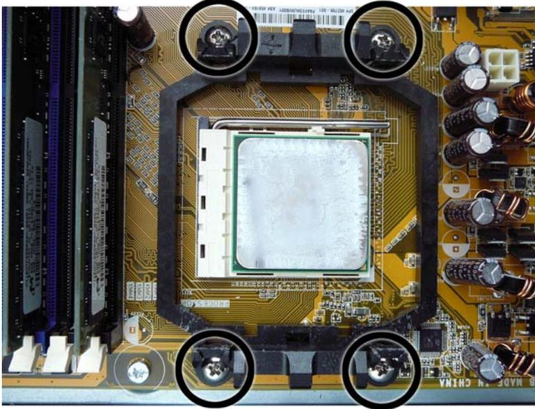
2. Remove the backplate from the system board.
