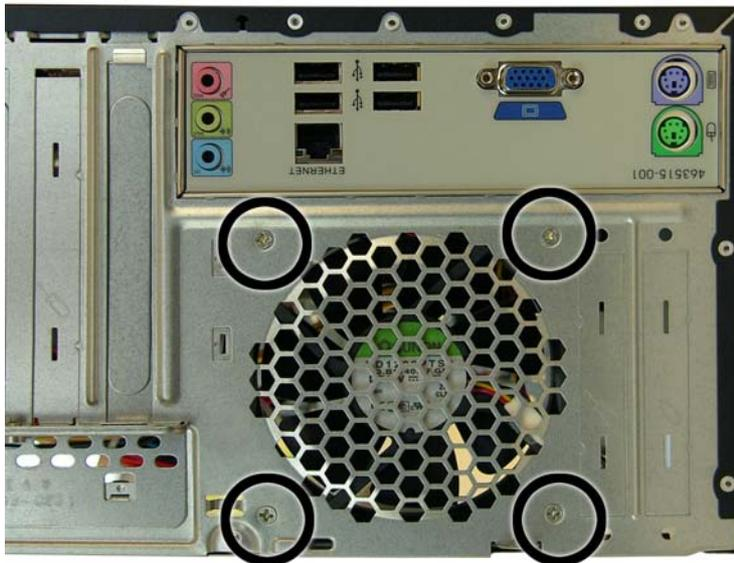
5. Lift the fan out of the chassis.
