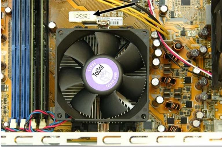
5. Pull the latch up so the metal hook rests above the tab on the backplate, and then press the latch toward the heatsink to disengage the metal hook on the opposite side of the heatsink from the backplate.
