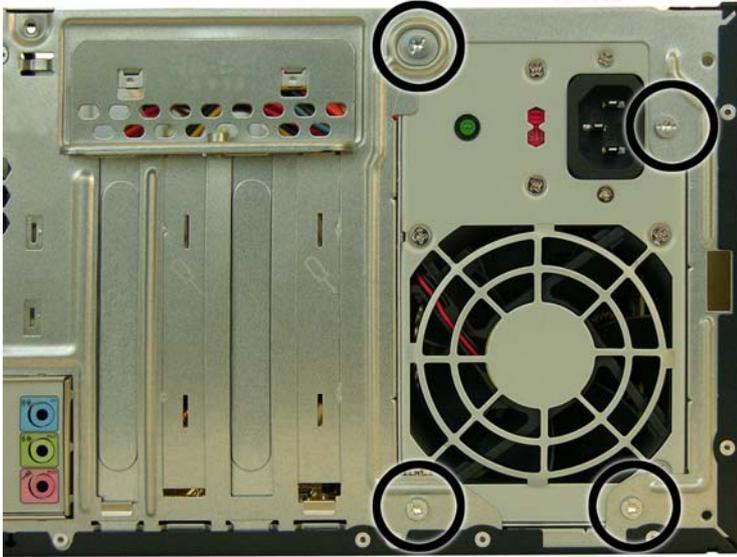
5. While pressing the tab in front of the power supply that holds it in place, pull the power supply up slightly to loosen it from the chassis.
