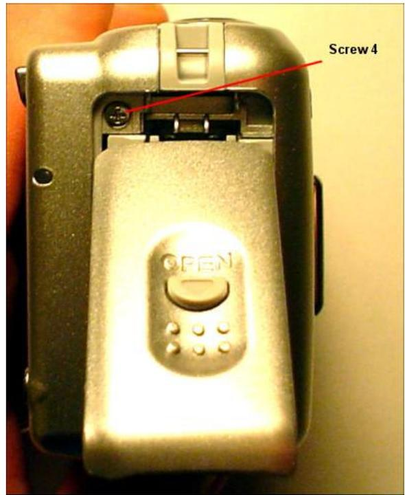
Remove screw 4 from under the battery door.
