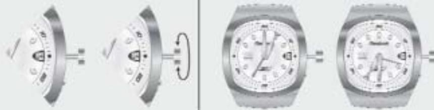
**3-Position Crown:** Pull crown to "MIDDLE" position and turn **CLOCKWISE** or **COUNTER-CLOCKWISE** until correct date appears.
