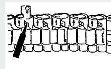
**Reassembly:** Rejoin bracelet parts. Push pin back into link in opposite direction of arrow. Press pin down securely into bracelet until it is flush.
