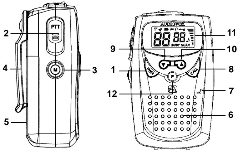
1. **Power Button (PWR):** Press and hold this button for 2 seconds to turn the transceiver on or off.
