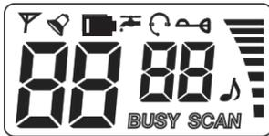
The FR-540 is equipped with an LCD display to indicate its settings and functions. When the radio is on, pressing any button will illuminate the display for 5 seconds.
