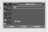
◆ When you connect equipment to the TV, you can choose between the following sets of jacks: "AV3", "S-Video2" on the TV's side panel or "AV1", "AV2", "S-Video1", "Component1", "Component2", "DVD" or "HDMI" on the TV's rear panel.
