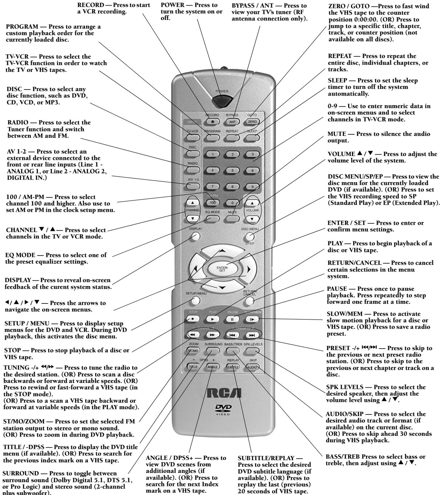
**NOTE: PROGRESSIVE SCAN** - To enable Progressive Scan, open the DVD disc tray and then press **STOP** 5 times (PSCAN ON appears on the front panel display). To return to Interlaced Scan mode, open the disc tray and press **STOP** 5 times (PSCAN OFF appears on the front panel display).
