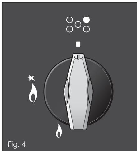
To turn the burner off, fully rotate the knob clockwise to the
