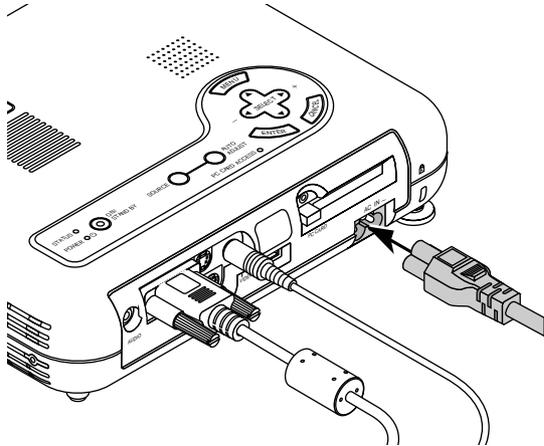
Plug the supplied power cable in the wall outlet. The projector will go into its standby mode and the power indicator will glow orange.
