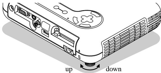
Do not use the tilt-foot for purposes other than originally intended. Misuses such as gripping the tilt-foot or hanging on the wall can cause damage to the projector.
