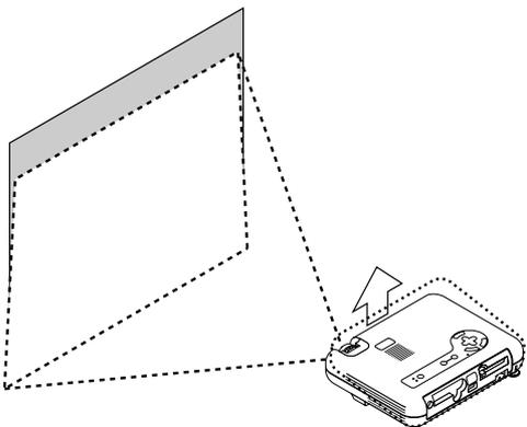
*Lift the front edge of the projector to center the image vertically.*
