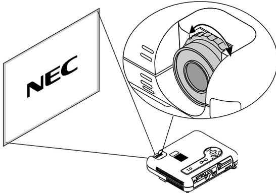
*Place your projector on a flat level surface and Ensure that the projector is square to the screen.*
