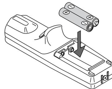
**3** Slip the cover back over the batteries until it snaps into place.
