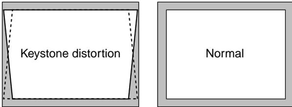
*NOTE: The maximum keystone angle that can be corrected is 45 degrees upward and 15 degrees downward with the projector placed horizontally on the ground plane.*
