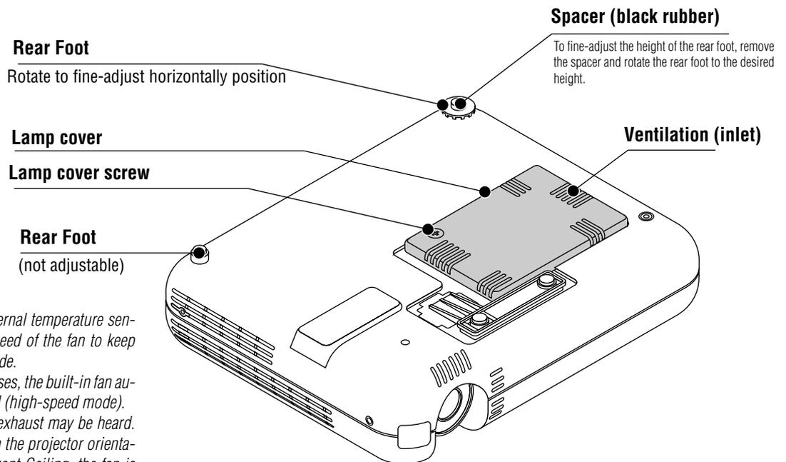
*NOTE: The projector has an internal temperature sensor. The sensor controls the speed of the fan to keep constant temperature in the inside. When the internal temperature rises, the built-in fan automatically runs at a high speed (high-speed mode). During this time, the sound of exhaust may be heard. This is not a malfunction. When the projector orientation is set to Rear Ceiling or Front Ceiling, the fan is automatically fixed at the high-speed mode.*
