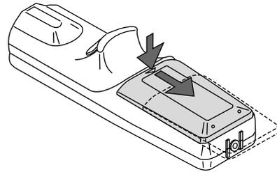
**2** Remove both old batteries and install new ones (AA). Ensure that you have the batteries' polarity (+/-) aligned correctly.
