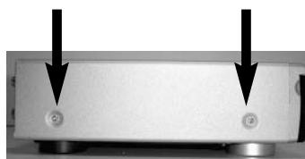
With the torx screwdriver, unscrew the two torx screws on the left-hand side of the unit.
