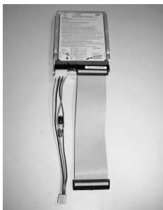
Attach the IDE cable and the power cable to your hard disk. Alternatively, you can do this after you have mounted the hard disk frames.
