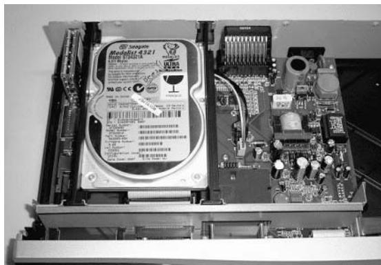
Insert the hard disk into the slot in the housing frame provided for the purpose, and lead the IDE cable and the power cable through below the hard disk.
