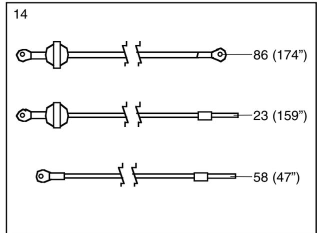
15. **Locate the Medium Cable (23).** Wrap the Medium Cable around a 3 1/2" Pulley (15). Attach the Pulley to the Top Frame (55) with a 3/8" x 3 3/4" Bolt (71) and a 3/8" Nylon Locknut (21). **Be sure that the end of the Cable with the ball is on the indicated side of the Pulley and that the Cable is between the Pulley and the hook.**
