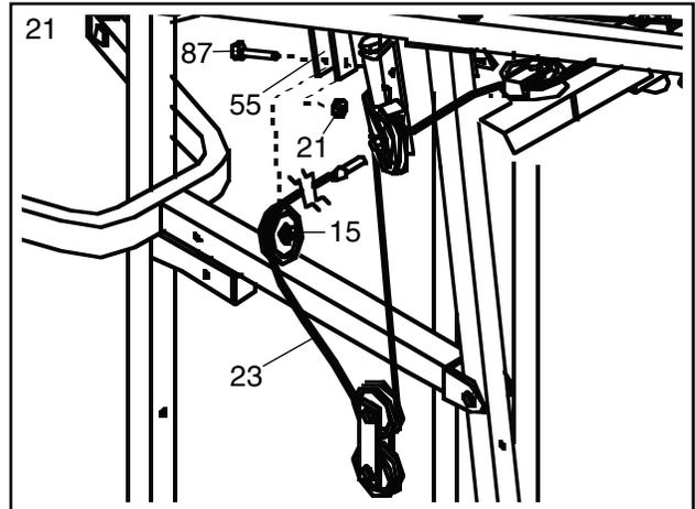
22. Wrap the Medium Cable (23) around a 3 1/2" Pulley (15). Attach the Pulley to the Top Frame (55) with a 3/8" x 1 3/4" Bolt (87) and a 3/8" Nylon Locknut (21).
