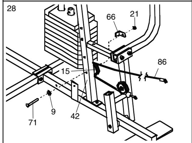
29. Wrap the Long Cable (86) around a 3 1/2" Pulley (15). Attach the Pulley and a Cable Trap (66) to the Press Frame (17) with a 3/8" x 3 1/2" Bolt (16), a 3/8" Flat Washer (9) and a 3/8" Nylon Locknut (21). **Be sure that the Cable Trap is turned to hold the Cable in place and that the Cable is routed around the Pulley as shown.**
