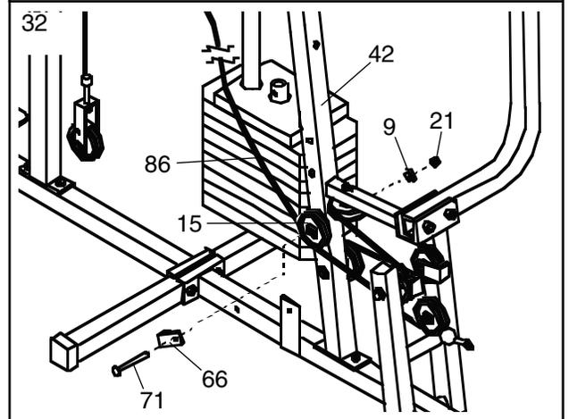
33. Route the Long Cable (86) over the lower 3 1/2" Pulley (15) attached to the "I"-Plates (81). The Cable must be routed from the direction shown.
