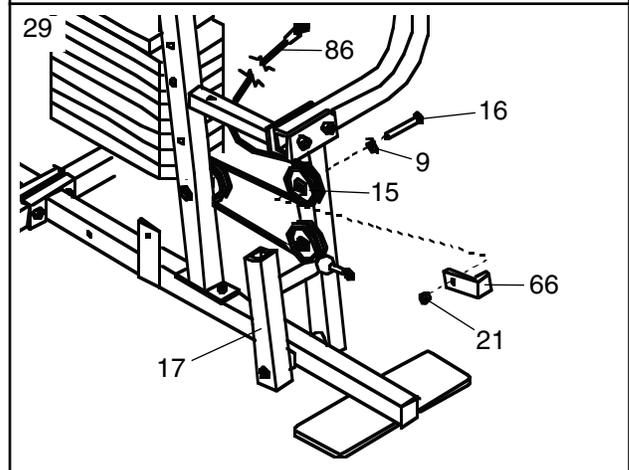
30. Wrap the Long Cable (86) around a "V"-Pulley (6). Attach the "V"-Pulley to the indicated hole in the Front Upright (42) with a 3/8" x 3 1/4" Bolt (85), a 3/8" Flat Washer (9), and a 3/8" Nylon Locknut (21). **Be sure that the Cable is in the groove of the "V"-Pulley and that the Cable is routed around the "V"-Pulley as shown.**
