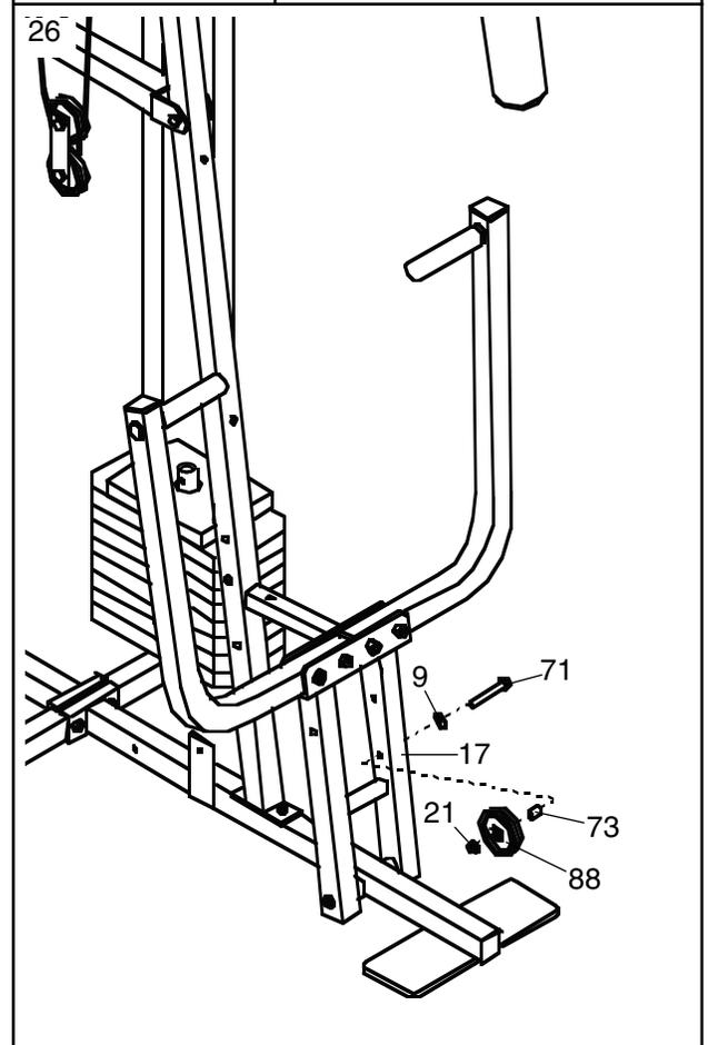
27. **Locate the Long Cable (86).** Route the Long Cable under the 3 1/2" Low Pulley (88). **Be sure that the end of the Cable with the ball is on the indicated side of the Press Frame (17) and that the Cable is between the Pulley and the crossbar on the Press Frame.** Tighten the 3/8" Nylon Locknut (21) and the 3/8" x 3 3/4" Bolt (not shown).
