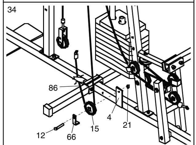
35. Route the Long Cable (86) around the indicated 3 1/2" Pulley (15) and through the Long "U"-Bracket (57). **The Cable must be between the Cable Trap (66) and the Pulley.** Tighten 3/8" x 2" Bolt (12) and the 3/8" Nylon Locknut (not shown). **Be sure that the Cable is in the groove of the Pulley and that the Cable and Pulley move smoothly.**
