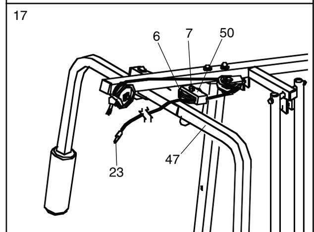
18. Route the Medium Cable (23) around the “V”-Pulley (6) on the Right Arm (48). **Be sure that the Cable is in the groove of the “V”-Pulley and that the Long Cable Trap (50) is turned to hold the Cable in place.** Tighten the 3/8” x 2 1/2” Bolt (7) and the 3/8” Nylon Locknut (not shown).
