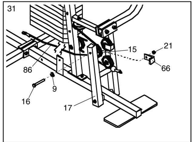
32. Wrap the Long Cable (86) around a 3 1/2" Pulley (15). Attach the Pulley and a Cable Trap (66) to the indicated hole in the Front Upright (42) with a 3/8" x 3 3/4" Bolt (71), a 3/8" Flat Washer (9), and a 3/8" Nylon Locknut (21). **Be sure that the Cable Trap is turned to hold the Cable in place and that the Cable is routed around the Pulley as shown.**
