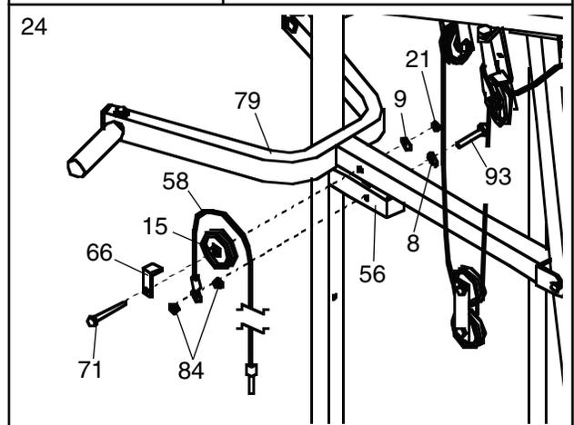
Wrap the Short Cable (58) around a 3 1/2" Pulley (15). Attach the Pulley and a Cable Trap (66) to the Squat Arm (79) with a 3/8" x 3 3/4" Bolt (71), a 3/8" Flat Washer (9), and a 3/8" Nylon Lock Nut (21). **The Cable Trap must be turned to hold the Cable in place.**
