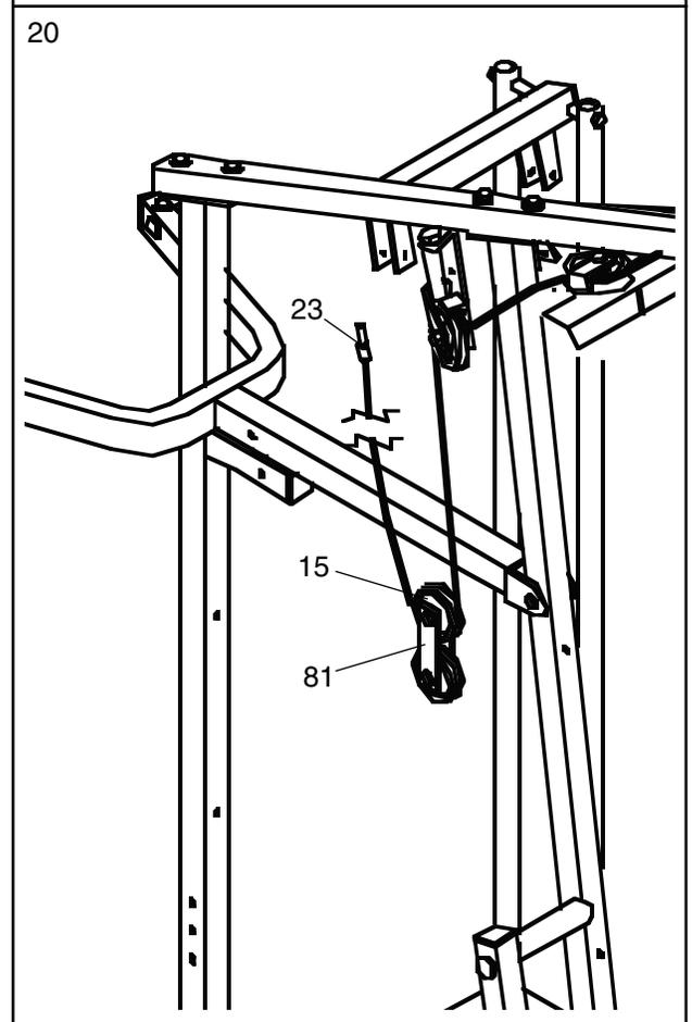
21. Wrap the Medium Cable (23) around a 3 1/2" Pulley (15). Attach the Pulley to the Top Frame (55) with a 3/8" x 1 3/4" Bolt (87) and a 3/8" Nylon Locknut (21).
