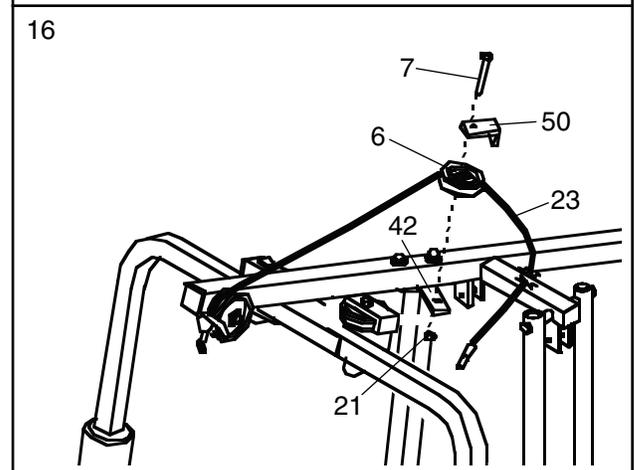
17. Route the Medium Cable (23) around the "V"-Pulley (6) on the Left Arm (47). **Be sure that the Cable is in the groove of the Pulley and that the Long Cable Trap (50) is positioned to hold the Cable in place.** Tighten the 3/8" x 2 1/2" Bolt (7) and the 3/8" Nylon Locknut (not shown).
